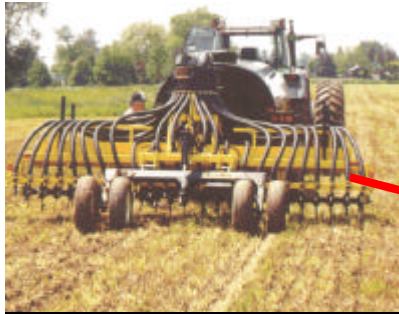
AERWAY Sub-Surface Deposition (SSD) manure applicator
